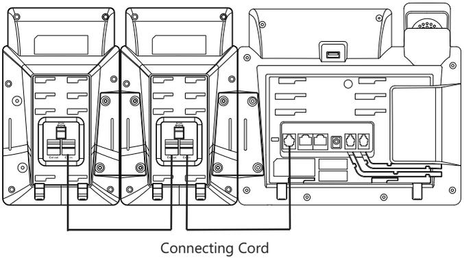
Note: You can connect six modules at most. You just need to connect the Ext in jack of the previous module and the Ext out jack of the next module using a connecting cord.
