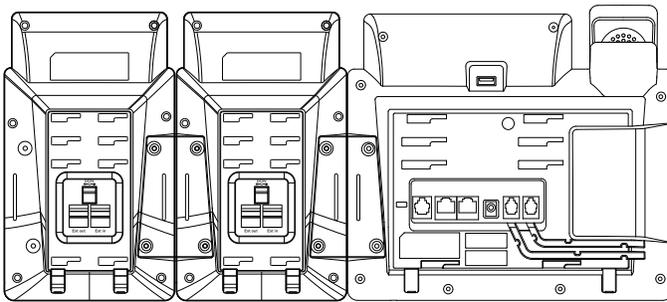
**Note:** The T48S/T48G/T46S/T46G IP phone can support six expansion modules at most. But if you use more than two expansion modules, you need to connect an additional power adapter to any one of the expansion modules.
