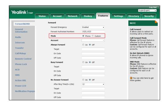
2. In the Forward block, mark the desired radio box in the Mode field.
